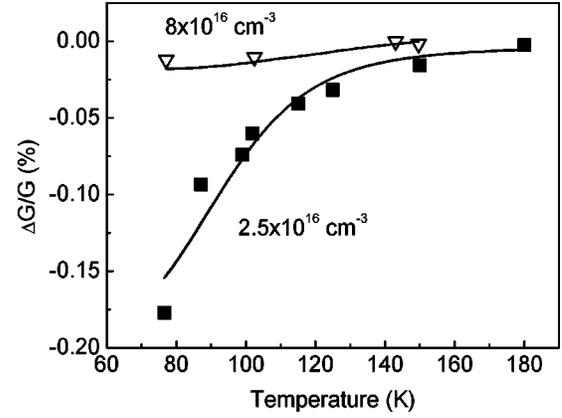
FIG. 4. Temperature dependence of the photoconductivity minimum for two SAQD's samples with different antimony concentrations  $N_{\text{epi}}$ . The solid lines refer to theory, as explained in text.
