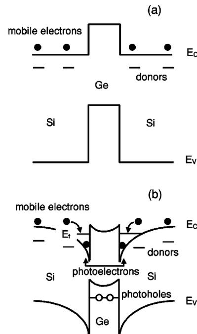
FIG. 1. Band structure of an *n*-type Ge/Si heterostructure with Ge SAQD's (a) in the absence of light and (b) under interband illumination. The figure illustrates the mechanism of negative interband photoconductivity. Potentials due to strain are not included.
