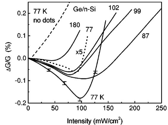
FIG. 3. Dependence of the relative photoconductivity on the interband illumination intensity in two  $n$ -type Si samples with Ge SAQD's (dot and solid lines) and in a sample without Ge nanoclusters (dashed line) at various temperatures. Solid lines correspond to antimony concentration  $N_{epi} = 2.5 \times 10^{16} \text{ cm}^{-3}$ , the dotted line corresponds to  $N_{epi} = 8 \times 10^{16} \text{ cm}^{-3}$ . Error bars indicate the typical uncertainty which applies to all curves.
