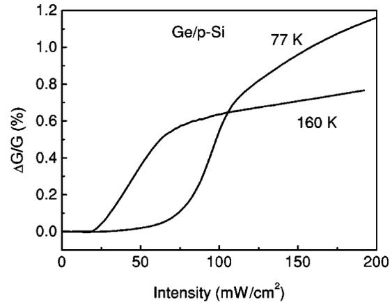
FIG. 5. Dependence of the relative photoconductivity on the interband illumination intensity in  $p$ -type Si with Ge quantum dots.
