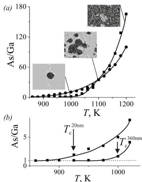
**Fig. 2** The temperature dependences of evaporated As/Ga ratio of two surface orientations ((111)A – squares, (111)B – circles) for  $L = 360$  nm (a), and different terrace width for the (111)A surface (b). Top views of the model surface in (a) correspond to  $T < T^*$ ,  $T = T^*$  and  $T > T^*$ .
