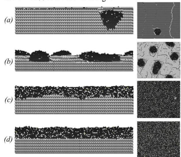
**Fig. 1.** Cross-sections and top views of GaAs model substrates (111)A (a, c) and (111)B (b, d) after the annealing at  $T = 1000$  K (a, b),  $T = 1200$  K (c, d). Liquid gallium is marked in black, solid Ga – in gray, As – in white colors.
