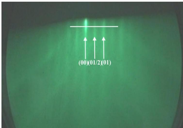
**Figure 3.** RHEED pattern from Si(100)  $2\times 1+1\times 2$  surface in [110] direction which was annealed 2 hours under temperature  $600^{\circ}\text{C}$ , then 30 minutes under  $700^{\circ}\text{C}$  and  $800^{\circ}\text{C}$  during 10 minutes.
