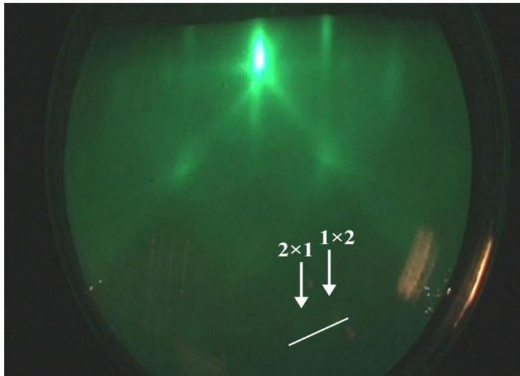
**Figure 2.** RHEED pattern from Si(100)  $2\times 1+1\times 2$  surface in [100] direction which was annealed under temperature  $1000^{\circ}\text{C}$  during 10 minutes in the low Si flux  $10^{13}$   $\text{at.cm}^{-2}\text{s}^{-1}$ .
