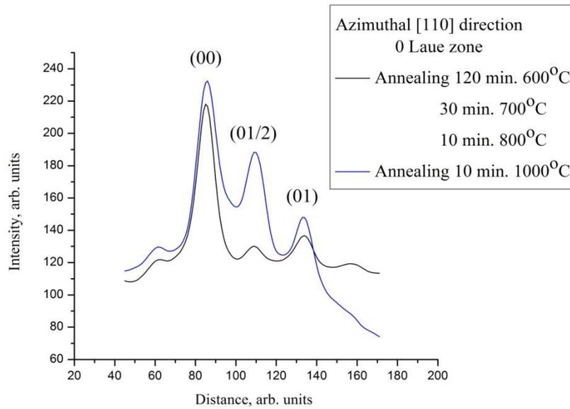
**Figure 6.** Profile along white line on RHEED pattern of the figure 3 and 4.
