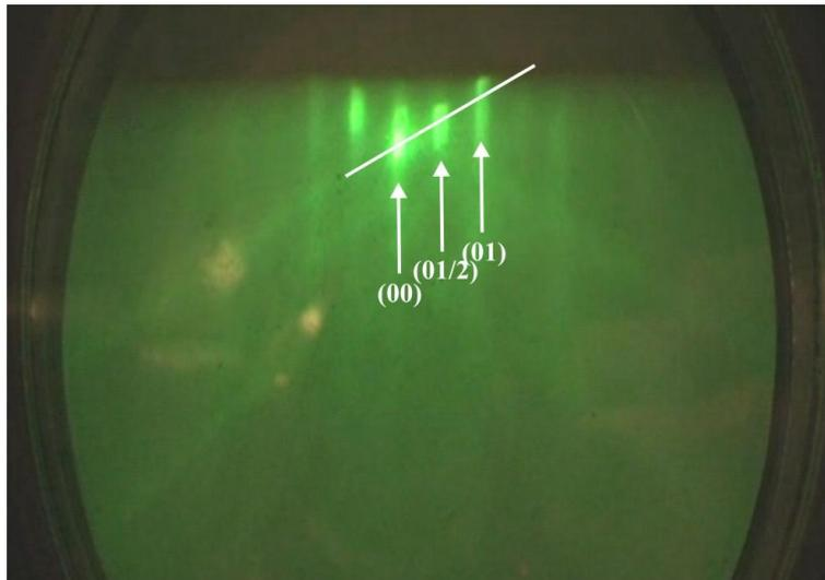
**Figure 4.** RHEED pattern from Si(100)  $2\times 1+1\times 2$  surface in  $[110]$  direction which was annealed under temperature  $1000^{\circ}\text{C}$  during 10 minutes in the low Si flux  $10^{13}$   $\text{at}\cdot\text{cm}^{-2}\cdot\text{s}^{-1}$ .
