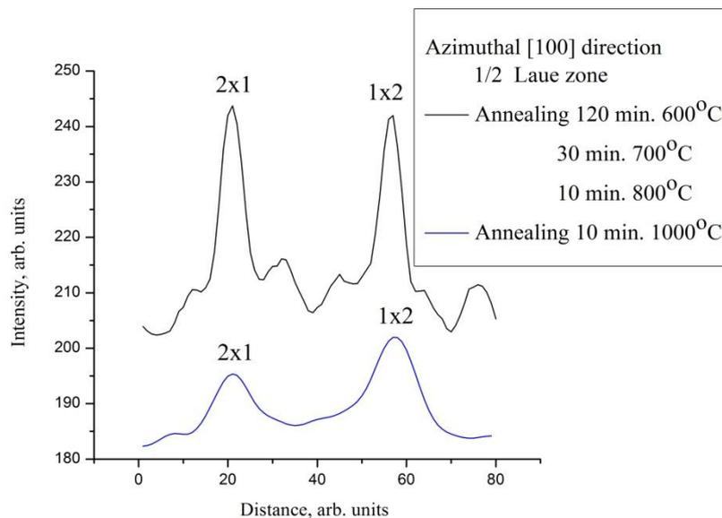
**Figure 5.** Profile along white line on RHEED pattern of the figure 1 and 2.
