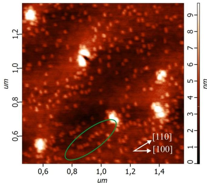
**Figure 7.** The Ge islands grown on Si(100) surface which was annealed 2 hours under temperature 600°C, then 30 minutes under 700°C and 800°C during 10 minutes.
