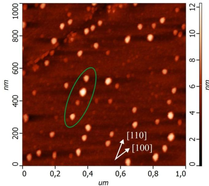
**Figure 8.** The Ge islands grown on Si(100) surface which was annealed under temperature  $1000^\circ\text{C}$  during 10 minutes in the low Si flux  $10^{13} \text{ at.cm}^{-2}\text{s}^{-1}$ .
