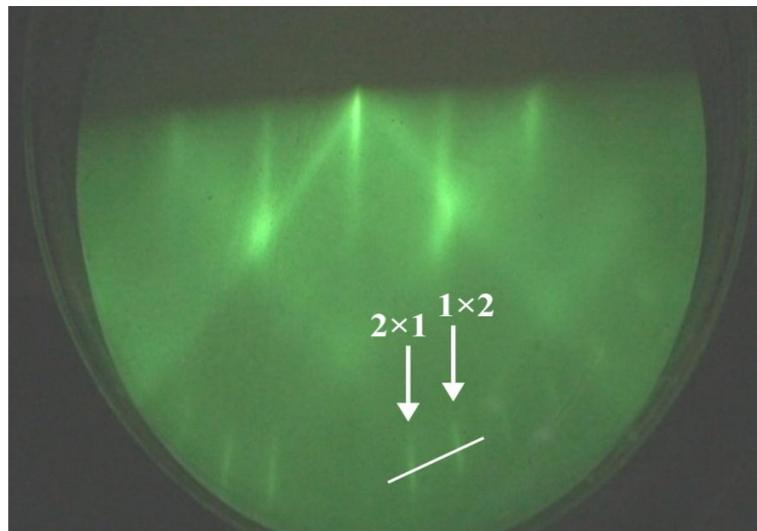
**Figure 1.** RHEED pattern from Si(100)  $2\times 1+1\times 2$  surface in [100] direction which was annealed 2 hours under temperature  $600^\circ\text{C}$ , then 30 minutes under  $700^\circ\text{C}$  and  $800^\circ\text{C}$  during 10 minutes.
